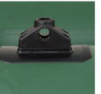
Begin by installing the side/deck mount into the glue on pads that are pre-installed on your Frameless Pontoon Boat. Be sure the "logo" on the mount reads upright when looking from inboard before securing the mount with the provided hardware.
