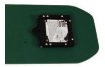
Using the included hardware, attach the seat mount to the predrilled holes on the floorboard. There are 2 sets of pre-drilled holes (6 holes in total). For the best performance we recommend using the first 4 pre-drilled holes closest to the front of the floorboard.
