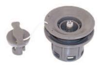
Recessed Air Valves Remove the cap and press and turn the valve stem counterclockwise so that the stem is in the UP position. Only when the stem is in this position the valve will retain air. Turning the stem clockwise will put the valve in the down position for deflation.
