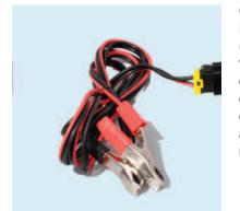
Connect the Turbo Pump to a 12V battery (car or marine) using the alligator clips at the end of the extension cord. Connect the red clip to the positive pole and the black clip to the negative pole.
