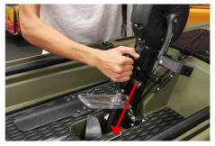
10. Make sure the fasteners are in same position as in image 8 before installing the drive. Move the propeller into vertical position and lower the drive into place.
