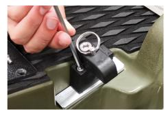
8. Screw in the 2 long screw into the inserts and screw tigh, using the allen key.
