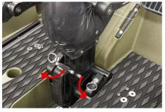
11. Lock the fasteners as shown above over the lower cylinders of the Drive. To remove the drive, make sure the propeller is in vertical position before raising the drive out of the well.
