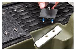
7. Put the aluminium plate with the screw holes closer to the wall as shown above.
