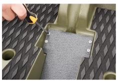
5. Use the phillips screw driver to remove the drive-well plate in the KingFisher,
