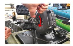
2. Fasten the pedals to the drive using the large allen key. Fasten tightly.
