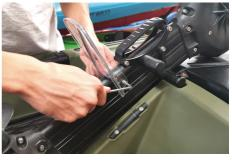
Attach the shield to the drive using the screw, washer and nut and tighten it with an allen key.
