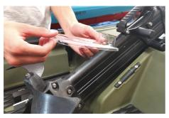
3. Fit the clear shield onto the drive as shown above, and align the screw hole on the shield with the one on the drive.
